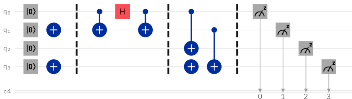
Figure 12. This is the encoded Bell State with a logical q_{0L} = |01\rangle composed of a physical q_0 and q_1 and a logical q_{1L} = |01\rangle composed of a physical q_2 and q_3 where we take |01\rangle to be our logical zero. The circle and plus sign without a target is the NOT gate and flips the qubit from one state to the other.
